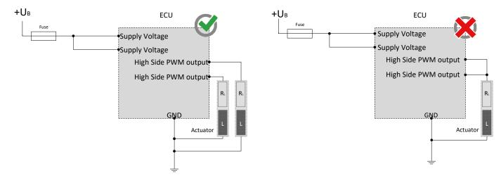
The pins (I/Os) can be used in combination and may not be switched externally against supply voltage.
